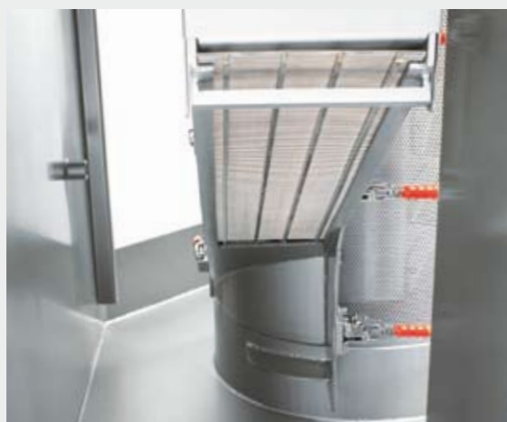
The prevention of dead spots, gaps and an off-peaking housing floor are the main features of the easy maintaining centrifugal dryer.
